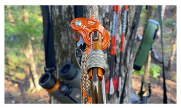
knot, it allows you to adjust your tether or lineman's rope length quickly with just one hand as opposed to two.
